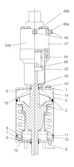
48a Valve connection 49a Supply air 49b Instrument air 50a Positioning type 73N-B 50b Positioning type 73N-F
