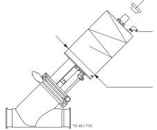
Max. 43.5 PSI (3 bar) "support air" on spring side.
