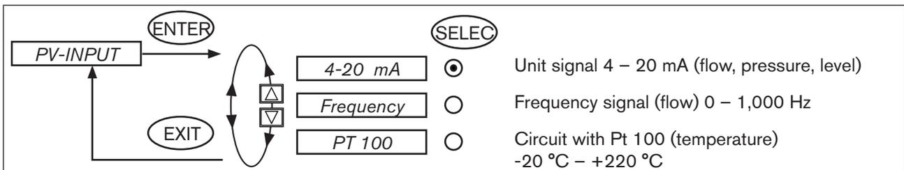
Figure 83: Operating structure P.CONTROL - PV-INPUT
