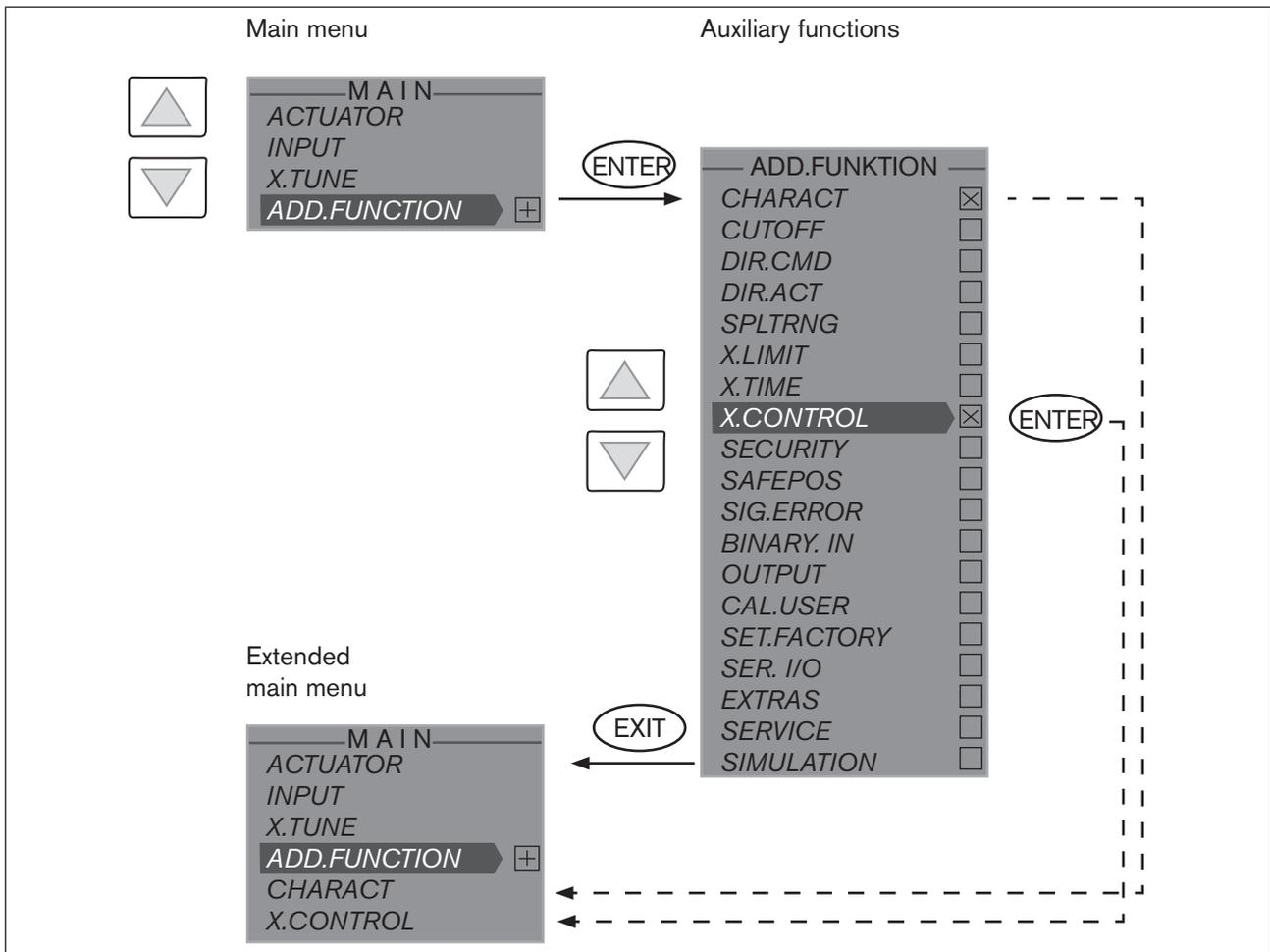
Figure 43: Including auxiliary functions
