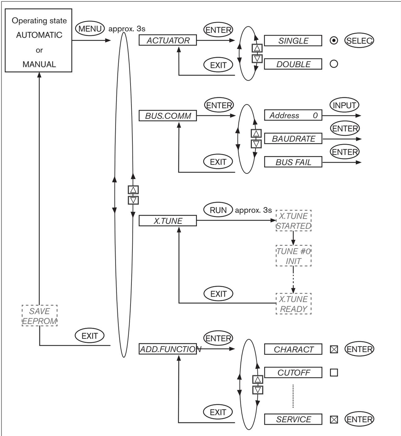
Figure 123: Operating structure of basic settings, DeviceNet
