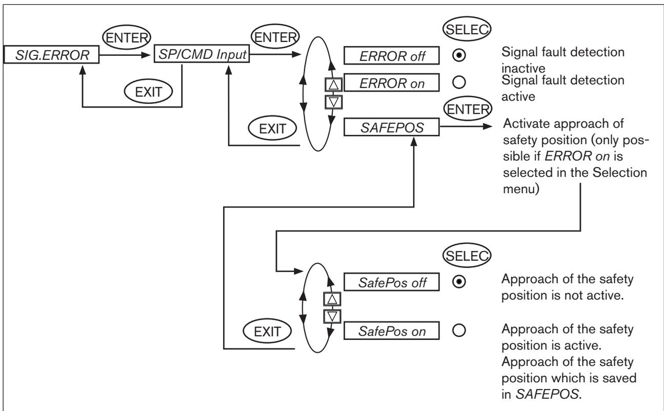
Figure 65: Operating structure SIG-ERROR
