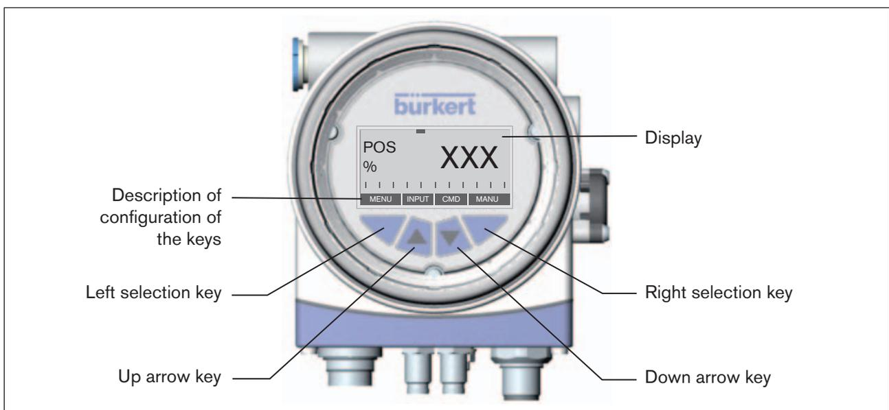
Figure 11: Description of the control module
