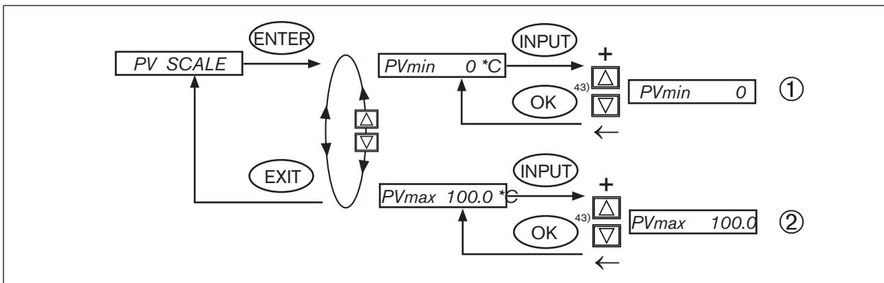
Figure 87: Operating structure P-CONTROL-PV-SCALE - Pt100
