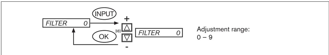
Figure 82: Operating structure P.CONTROL - FILTER
