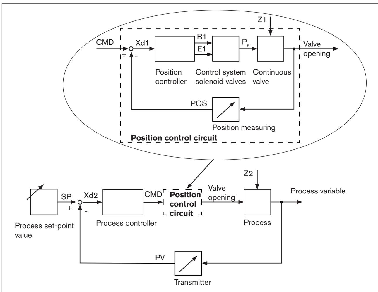
Figure 6: Signal flow plan of process controller
