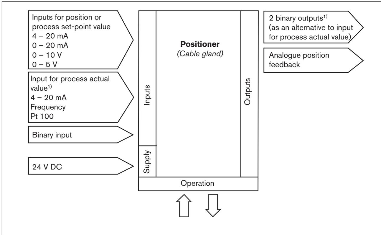
Figure 9: Interfaces for the model with cable gland
