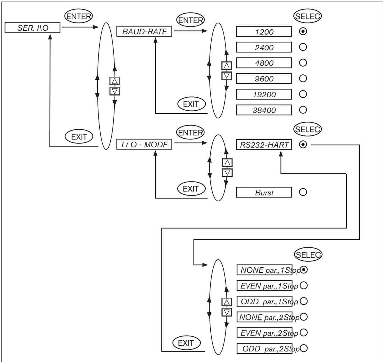
Figure 72: Operating structure SER. I/O
