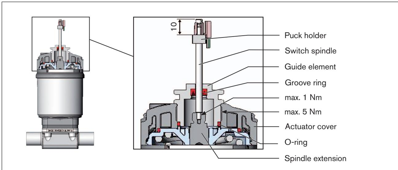
Figure 15: Installation of the switch spindle (2), series 2103, 2300 and 2301
