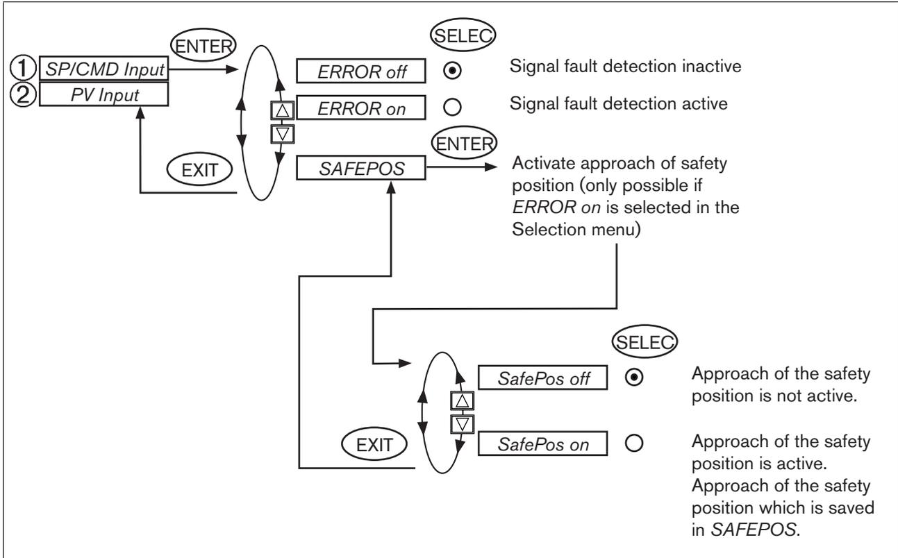
Figure 100: Operating structure SIG-ERROR-8693-SP-CMD-PV
