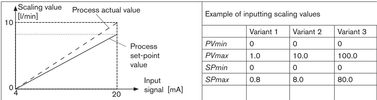
Figure 85: Scaling example
