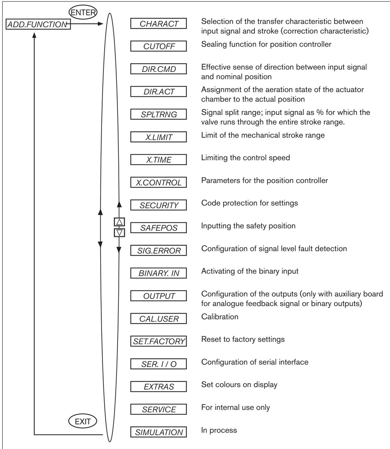
Figure 44: Overview - auxiliary functions, position controller Type 8692
