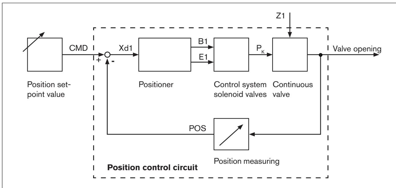
Figure 4: Signal flow plan of position controller
