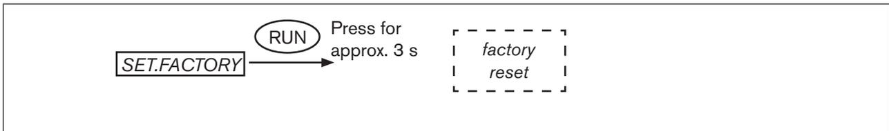
Figure 71: Operating structure SET.FACTORY
