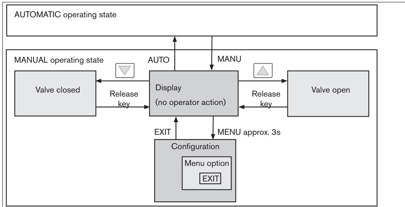
Figure 94: Operating structure MANUAL
