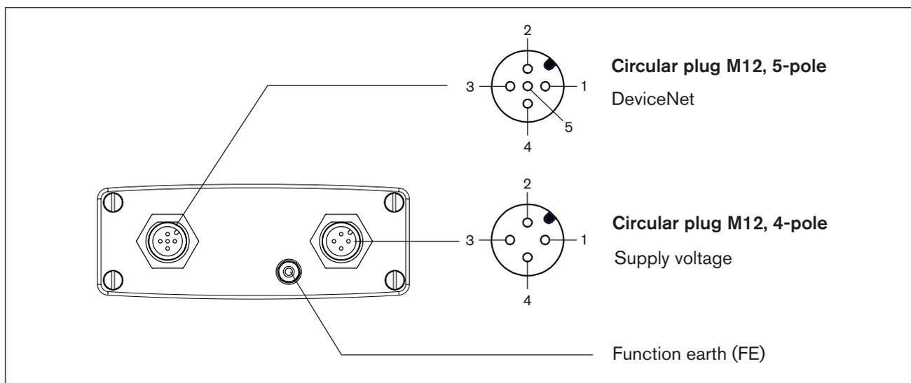
Figure 119: Connection of DeviceNet - Type 8692
