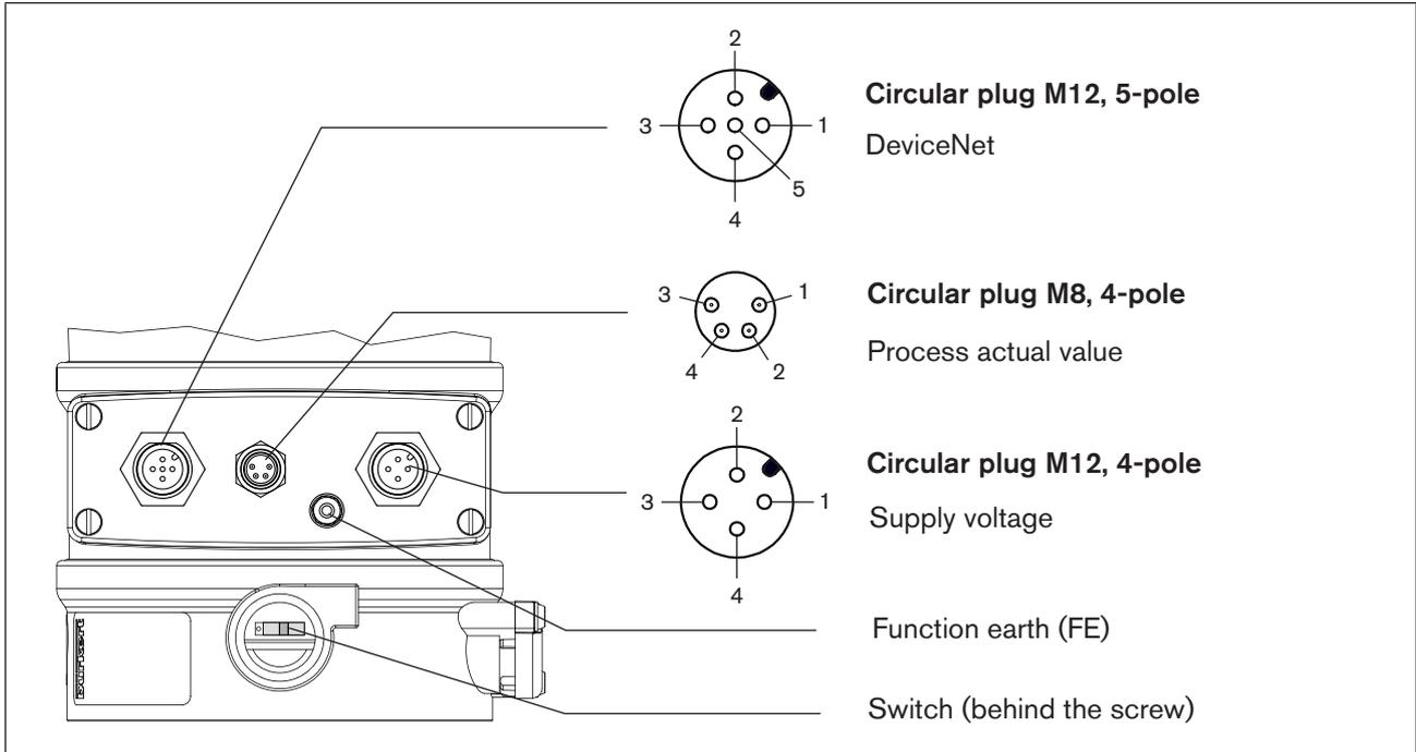
Figure 120: Connection of DeviceNet - Type 8693
