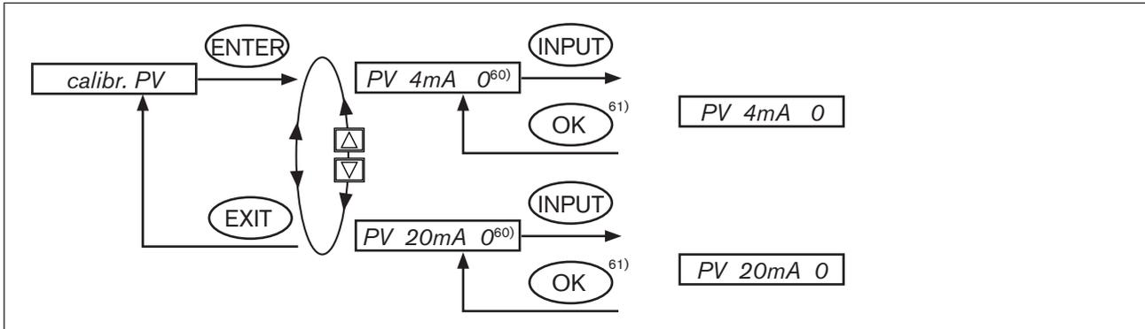
Figure 105: Operating structure CAL.USER-8693-PV-4-20
