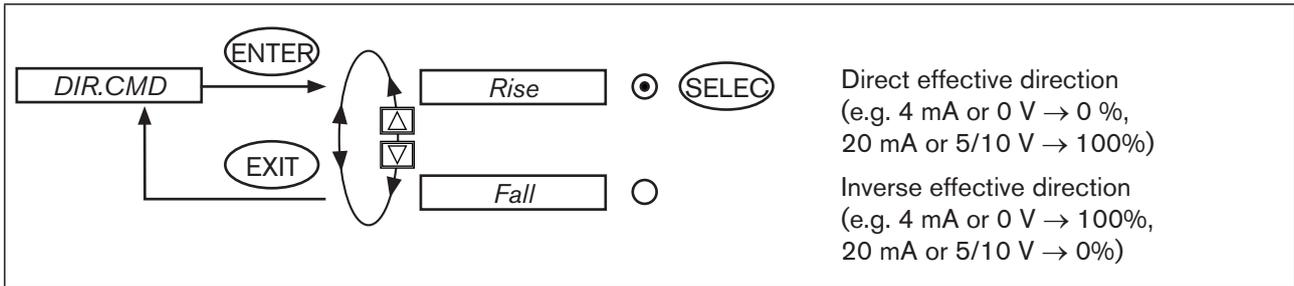
Figure 51: Operating structure DIR.CMD
