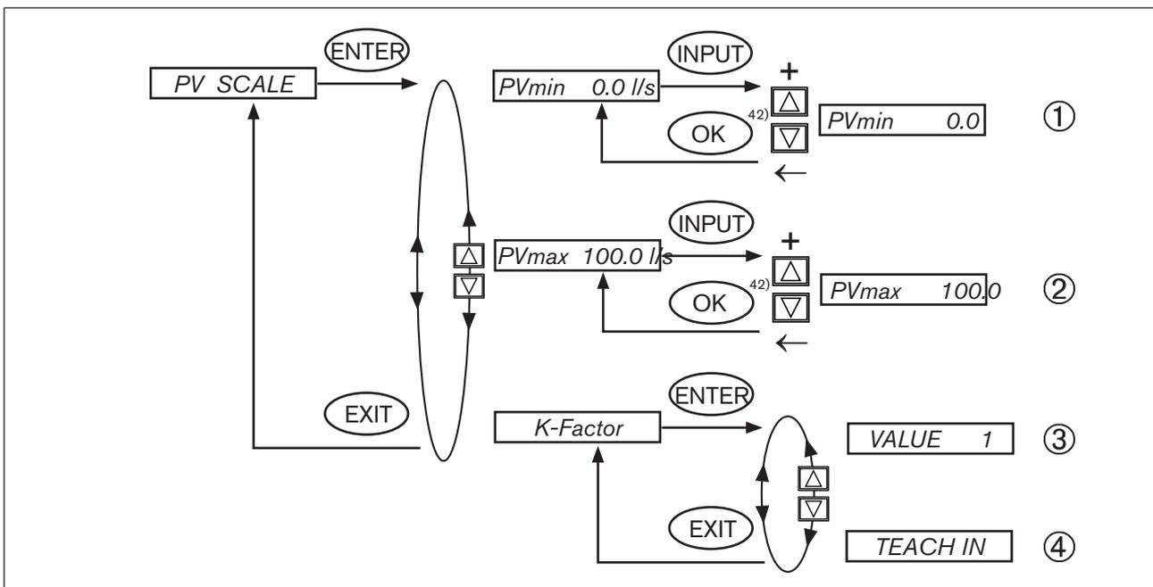
Figure 86: Operating structure P.CONTROL - PV-SCALE - Frequency
