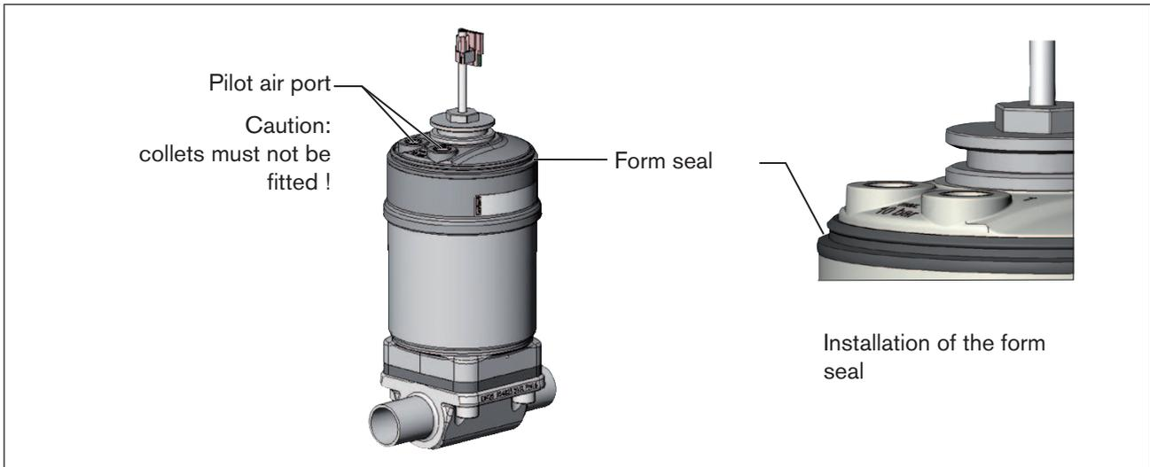
Figure 16: Installation of the sealing rings, series 2103, 2300 and 2301
