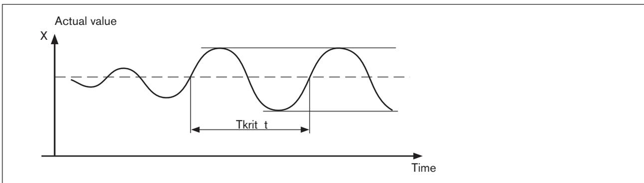
Figure 138: Progress of the control variable PID
