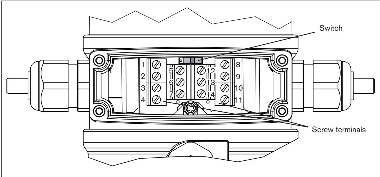
Figure 31: Terminal board with screw terminals and switch
