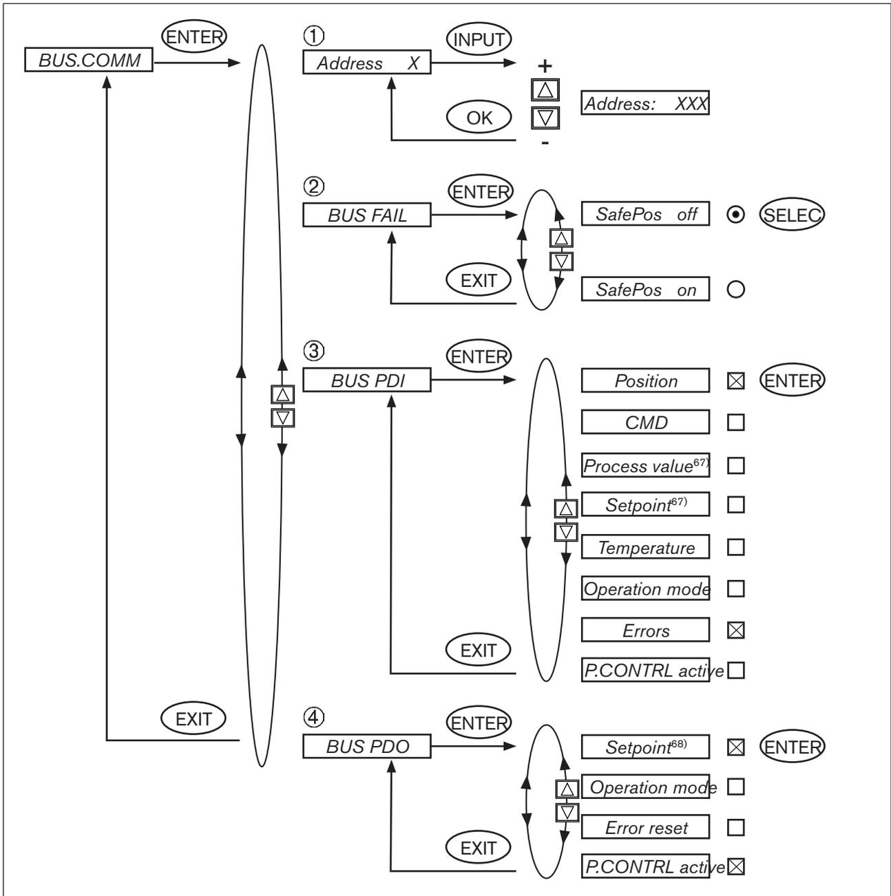
Figure 114: Operating structure - BUS-COMM - 8693
