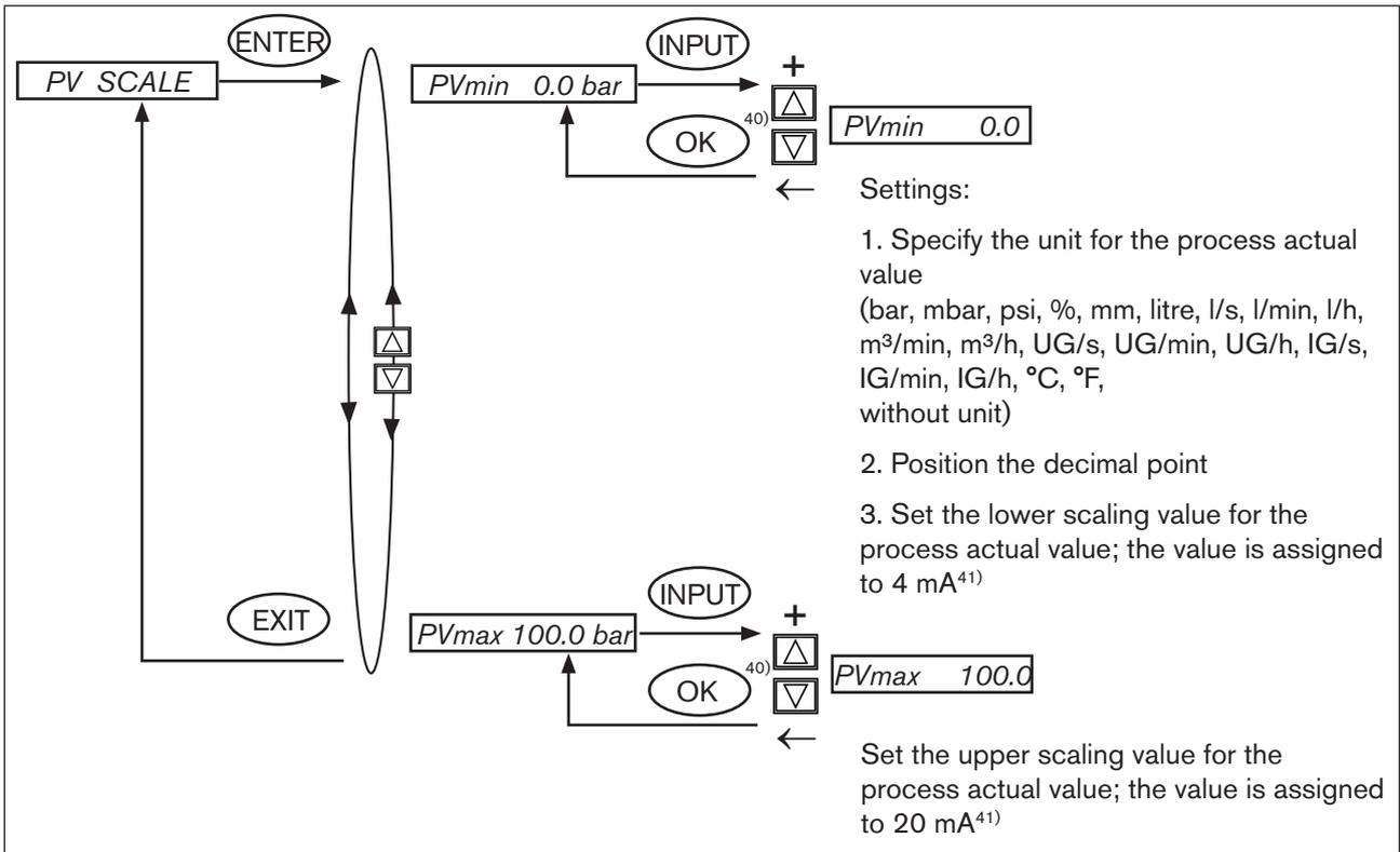
Figure 84: Operating structure P.CONTROL - PV-SCALE - 4-20mA
