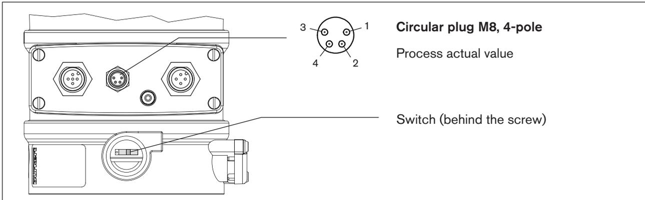
Figure 121: Connection DeviceNet - Process actual value - Type 8693
