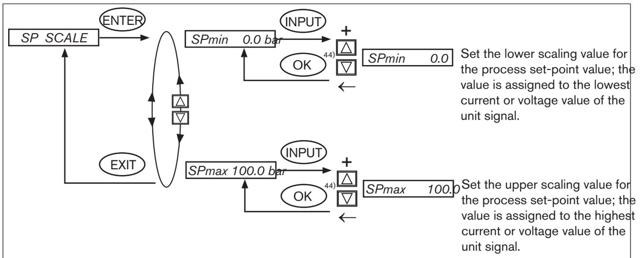
Figure 89: Operating structure P.CONTROL - SP-SCALE
