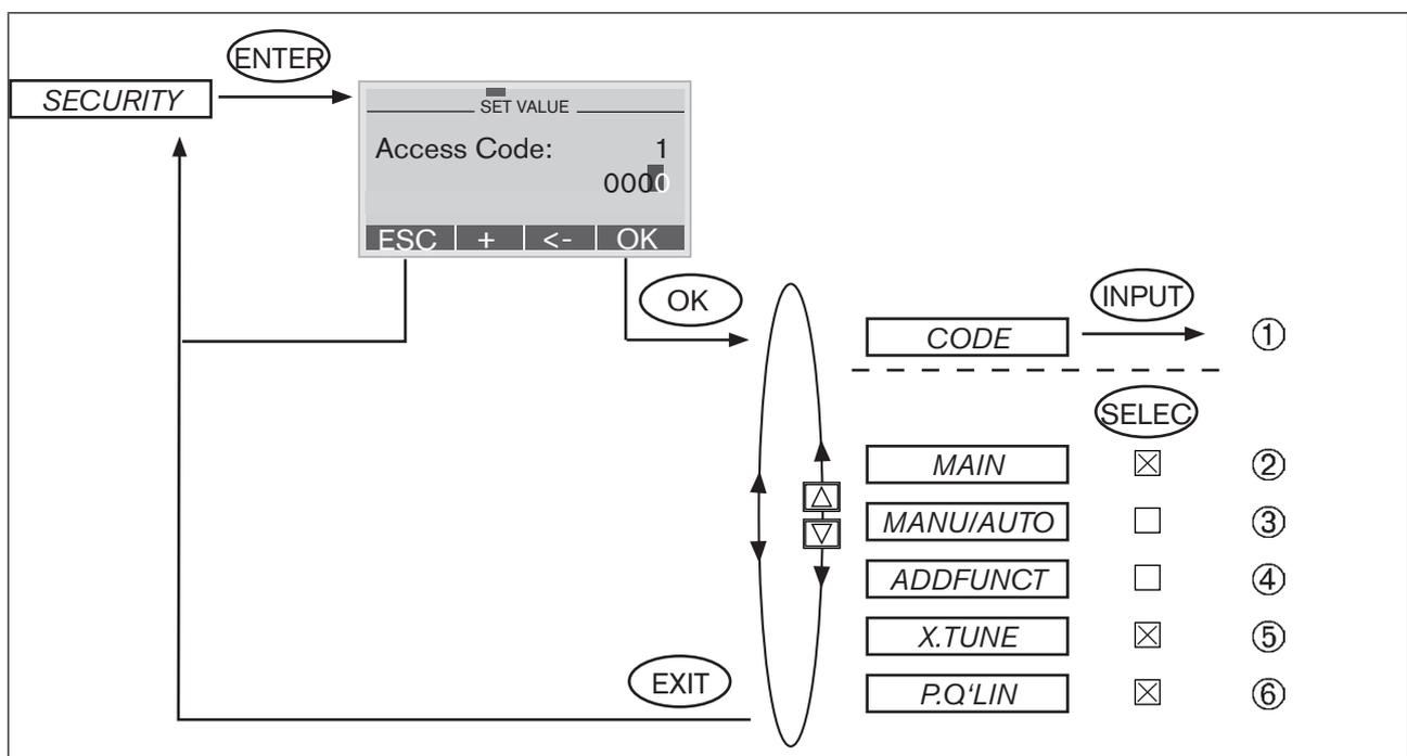
Figure 98: Operating structure SECURITY - 8693
