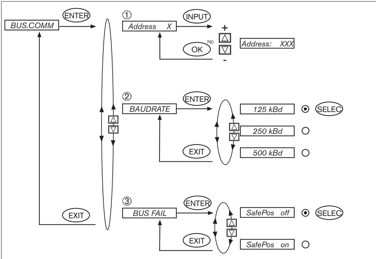
Figure 124: Operating structure - BUS-COMM - DeviceNet
