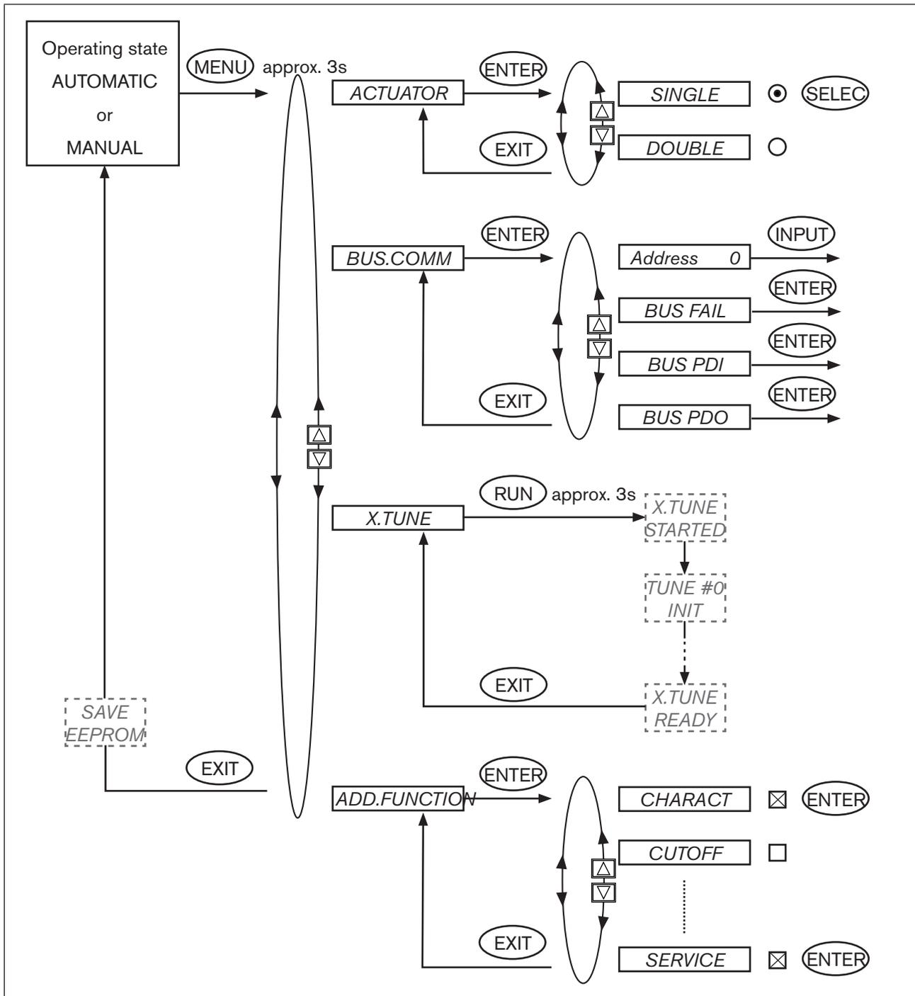
Figure 112: Operating structure - basic settings - PROFIBUS-DP
