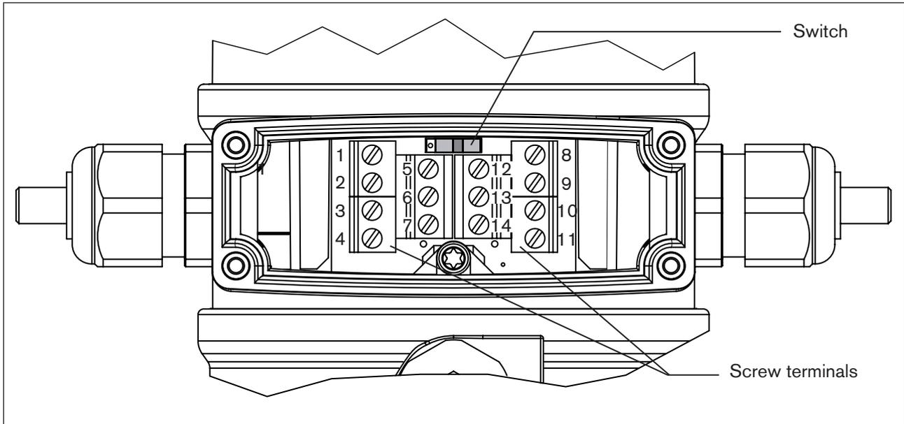
Figure 32: Terminal board with screw terminals and switch
