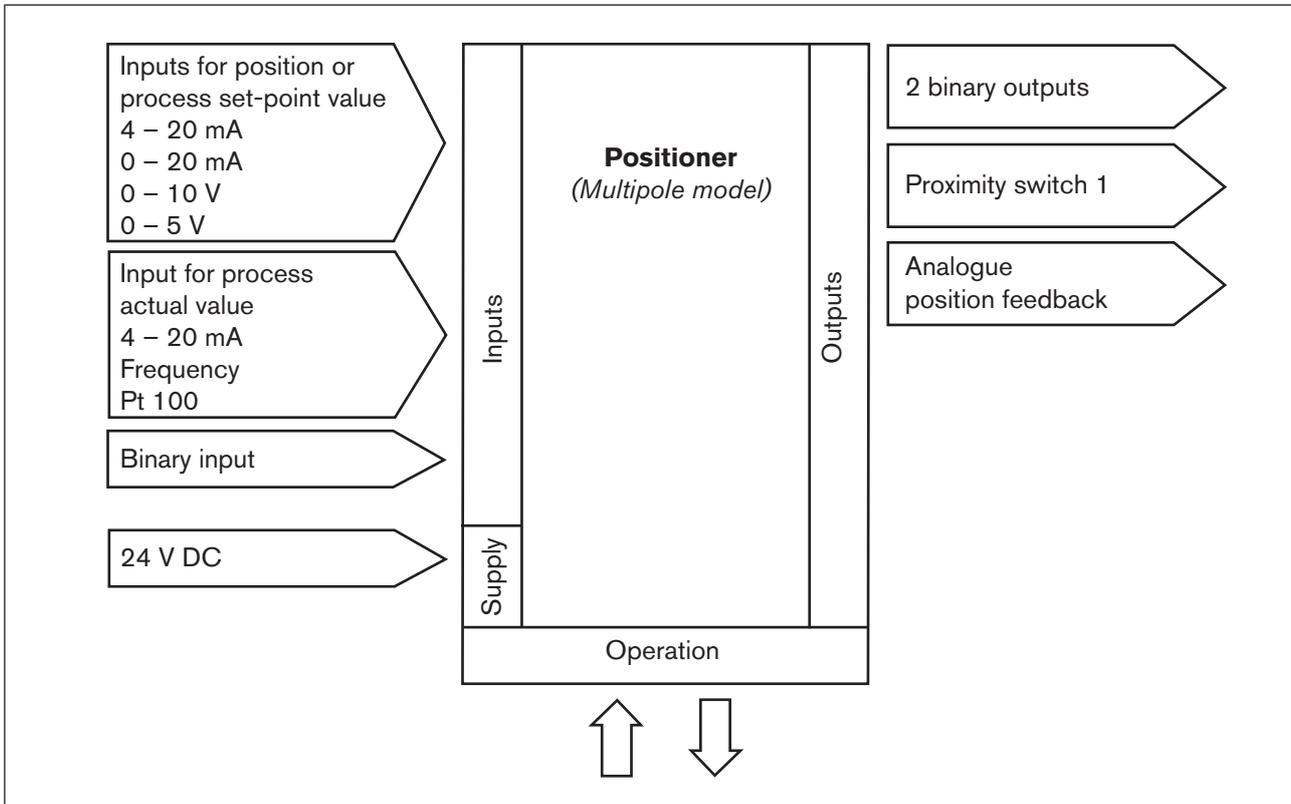
Figure 8: Interfaces for the multipole model
