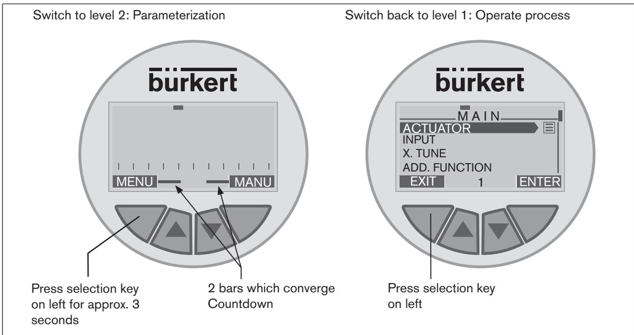
Figure 13: Switch operating level
