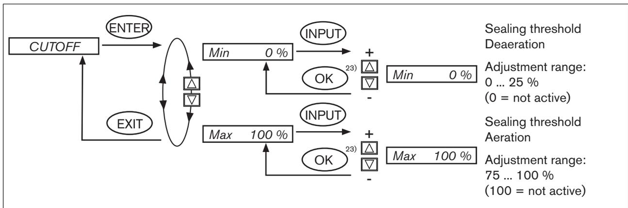
Figure 49: Operating structure CUTOFF
