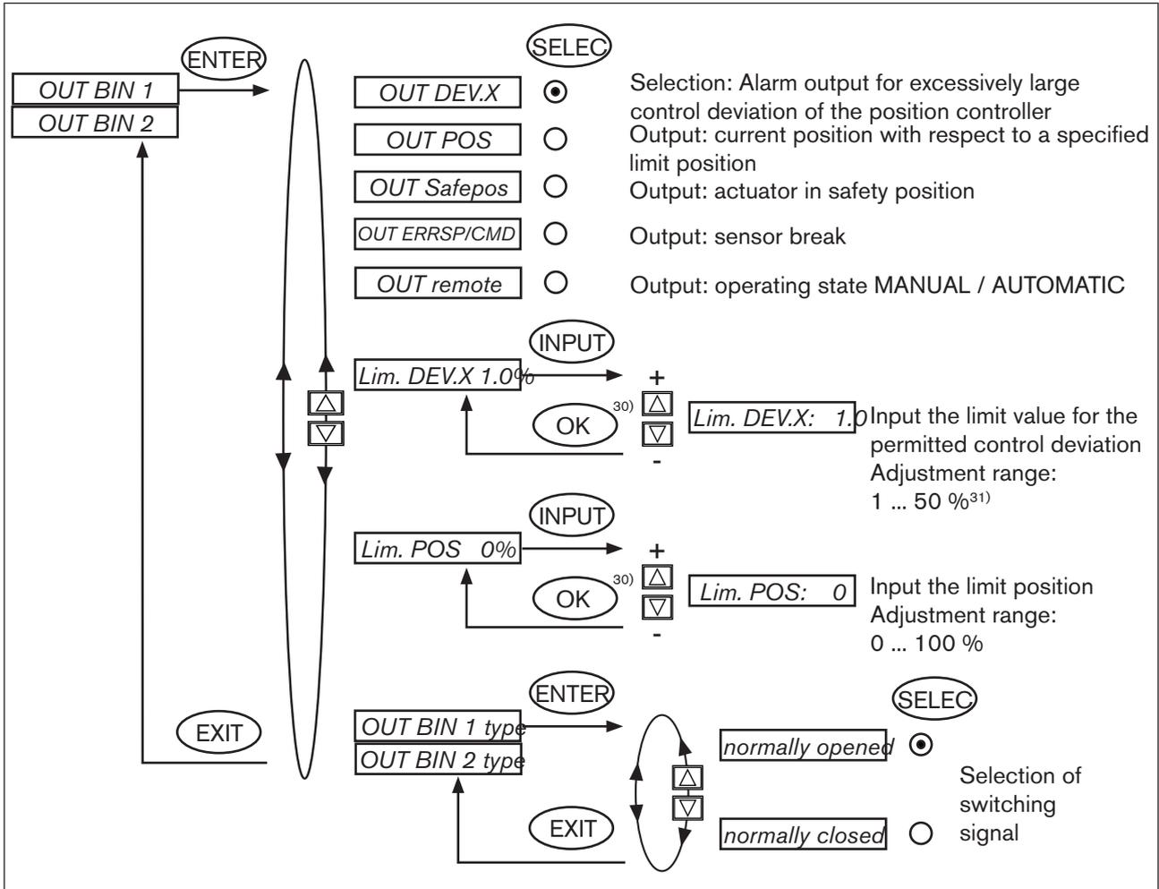
Figure 69: Operating structure OUTPUT-BIN1
