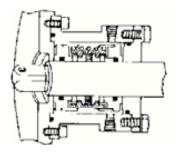
Type E is designed to withstand heavy duty vacuum applications (to 28" Hg), tacky products, slurries, or pumped products which may exceed 212°F. The seal chamber can be pressurized to permit use of drain piping for coolants
