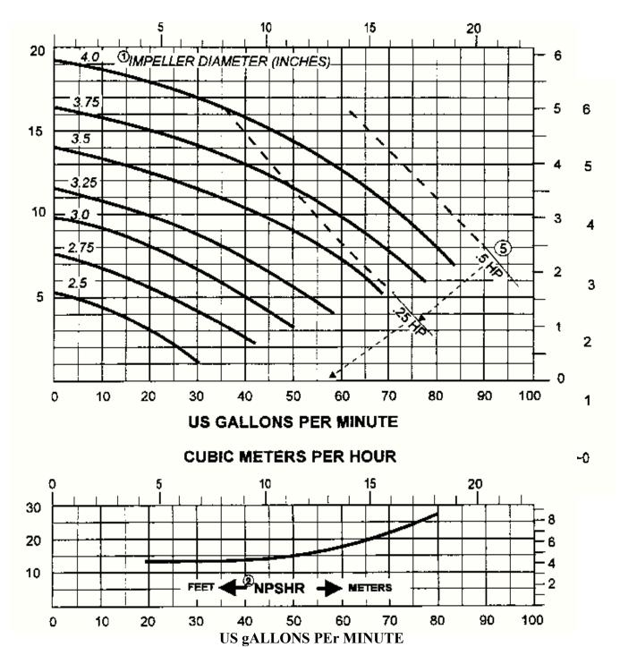
**NOTES:**Impeller diameters available in 1/16-inch increments Kg/cm = Head in Meters X Speçific Gravity
